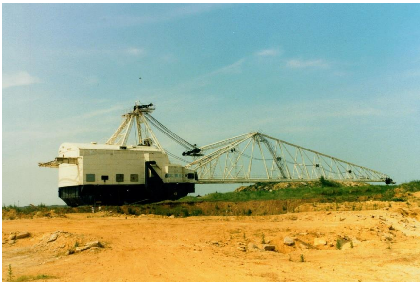
Figure 3. One of the Sundew draglines, a large electrically powered dragline excavator latterly used in mining operations in Corby's ironstone quarries.
