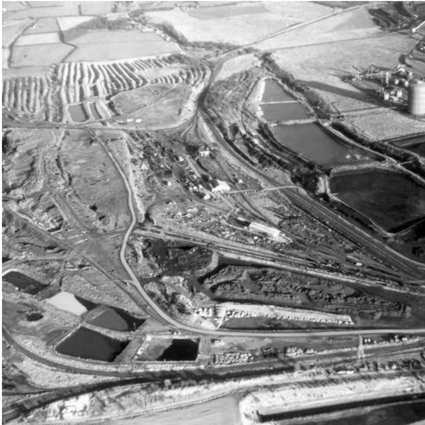
Figure 2. Aerial view of ironstone workings in the Corby region, with an area at the top of the photograph of the characteristic 'Hills and Dales' terrain left after open-cast mining.
